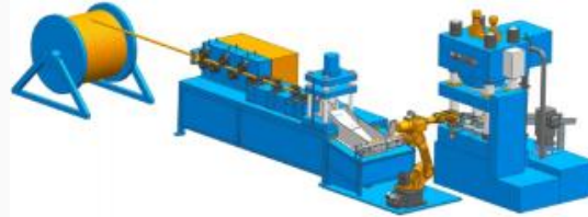
油压机上下料机器人布局图 Layout of feeding and discharging robot for hydraulic press
