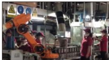
搬运机器人-黑茶砖 Carrying robot-black tea brick
