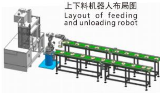
油压机上下料机器人布局图 Layout of feeding and discharging robot for hydraulic press
